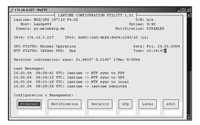
In addition to the SNMP and web interface, you can also manage your LANTIME configuration via a command line interface (CLI), which can be used via a TELNET or SSH connection. A setup tool can be started after login, just type "setup" and press ENTER at the prompt.
