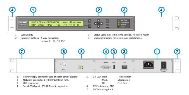
The implemented NTPD distributes the reference time from the receiver. Information on the NTPD is monitored on the LC display or can be inquired via the network.
