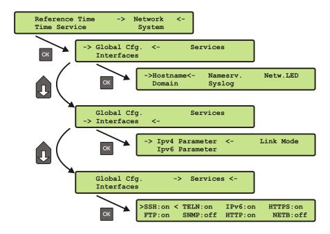
In this submenu the network configuration parameters related to the network interfaces can be changed. The submenus can be selected with the arrow keys and the "OK" button:
