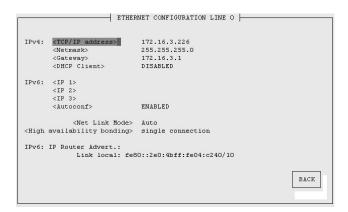
Here, the parameters for the network port can be changed. In the upper section of the page you can enter the IPv4 parameters, the lower part gives you access to the IPv6 parameters of the interface.
