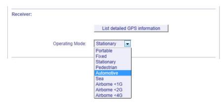
The example shows the menu with a GPS receiver and MGR module. With the button "List detailed GPS information" you can open a text field with all relevant receiver information. A LANTIME server with GPS receiver and MGR module can be adjust to its operational mode (appropriate environment) - computing the position to the expecting speed.
