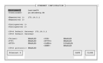
In the network configuration all parameters related to the network interfaces can be changed. In the first section you can change the hostname and domain name. You can also specify two nameservers and two SYSLOG servers. In the nameserver and SYSLOG server fields you may enter an IPv4 or IPv6 address (the SYSLOG servers can be specified as a hostname, too).
